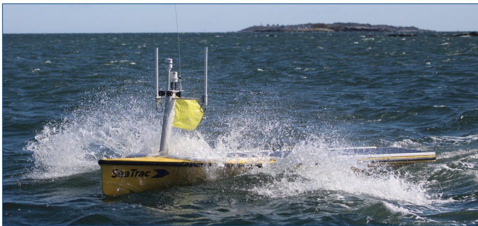
(Left) The SeaTrac SP-48 USV can perform shallow-water surveys in open ocean. (Below) Survey route.
